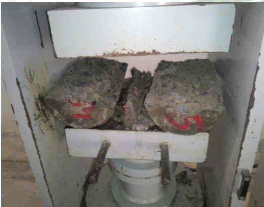
Fig. 2. Split tensile strength.
