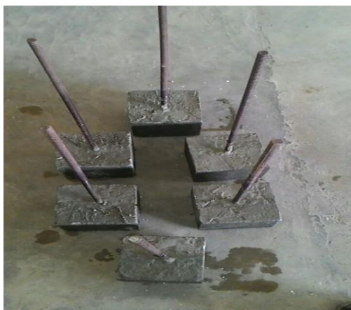
Fig. 6. Pull out test set up.
