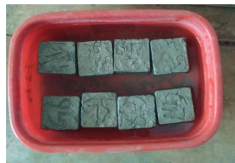
Fig. 4. Water absorption test.
