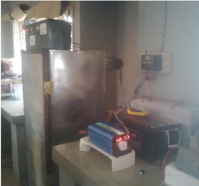
Plate. 4. View of the Synchronization of the Constructed Egg Incubator with the Installed Solar powered System in Operation.
