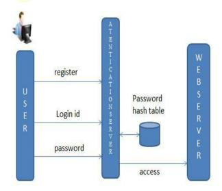
Fig. 1. Traditional password based system.
