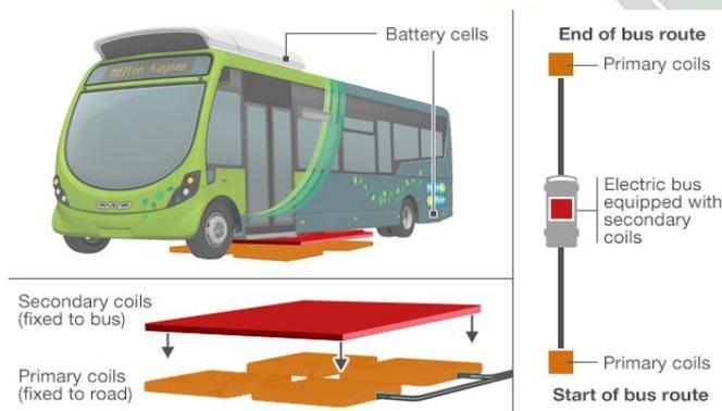
Fig. 1. Pollution free bus structure with inductive coupling.
