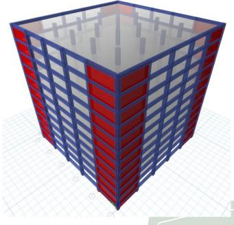
Fig. 6. 3D model of flat plate with both edge beam & shear wall.
