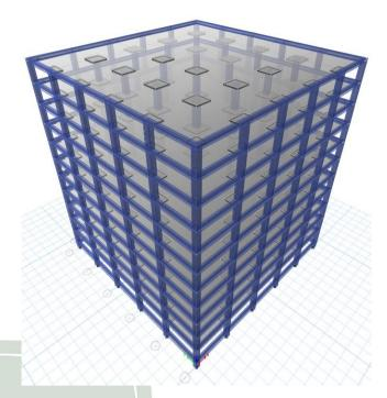
Fig. 8. 3D model of flat slab with edge beam & without shear wall.
