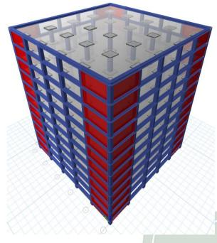
Fig. 10. 3D model of flat slab with both edge beam & shear wall.
