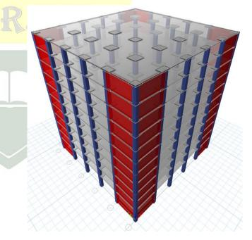
Fig. 9. 3D model of flat slab without edge beam & with shear wall.
