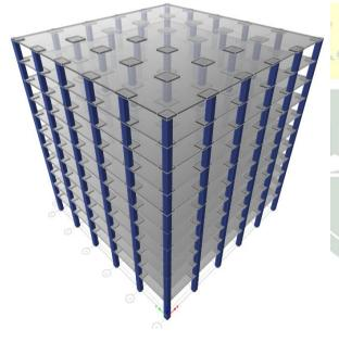
Fig. 7. 3D model of flat slab without edge beam & without shear wall.
