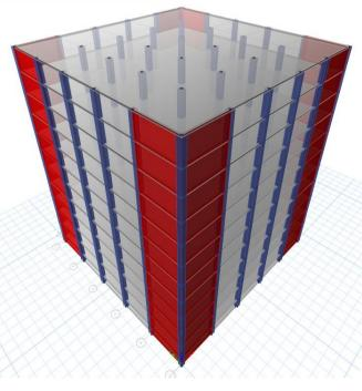
Fig. 5. 3D model of flat plate without edge beam with shear wall.
