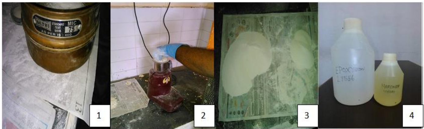
Fig. 1. (1) 75 \mu Sieve (2) Grinding of eggshells (3) Egg shell powder (4) Epoxy resin
