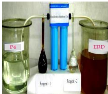
Fig. 10. Nanofiltration set up (ERD: Effluent after reactive colour dyeing and P4: permeate obtained after dyeing of jute was completed with 3 rd permeate)
