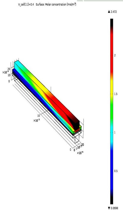
Fig.6. Cathode oxygen concentration at 493K
