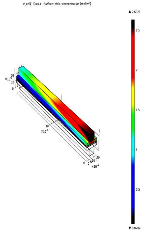
Fig.3. Cathode oxygen concentration at 463K
