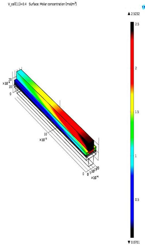
Fig.5. Cathode oxygen concentration at 483K
