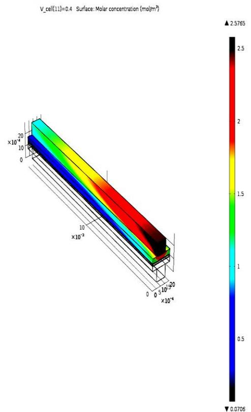
Fig.4. Cathode oxygen concentration at 473K
