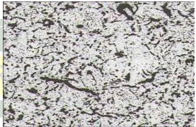
Fig.(3)Microstructure of Homogenized Alloys with (30)hrs. At 410 C°(45 m\mu )
