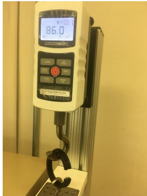
Figure 2: Stress testing machine measuring the breakpoint of a polypropylene tank mount part.
