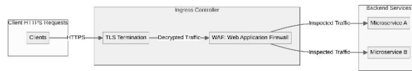
Fig. 1. Proposed Architecture for Securing Ingress Traffic with TLS Termination and WAF Integration.
