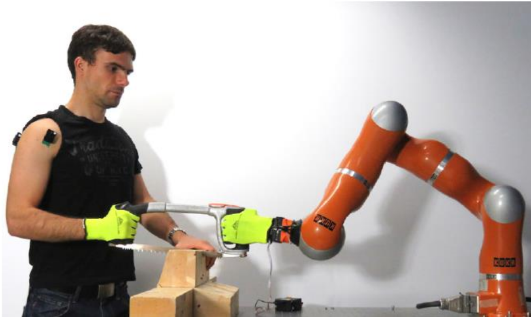
Fig. 4 human–robot manipulation framework for robot adaptation to human fatigue. Source: [10]
