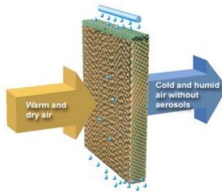
FIGURE 1: Direct Evaporative Cooling system
