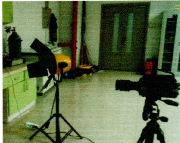
(c) High speed camera system Figure 3 Rolling Friction Coefficient Test Device
