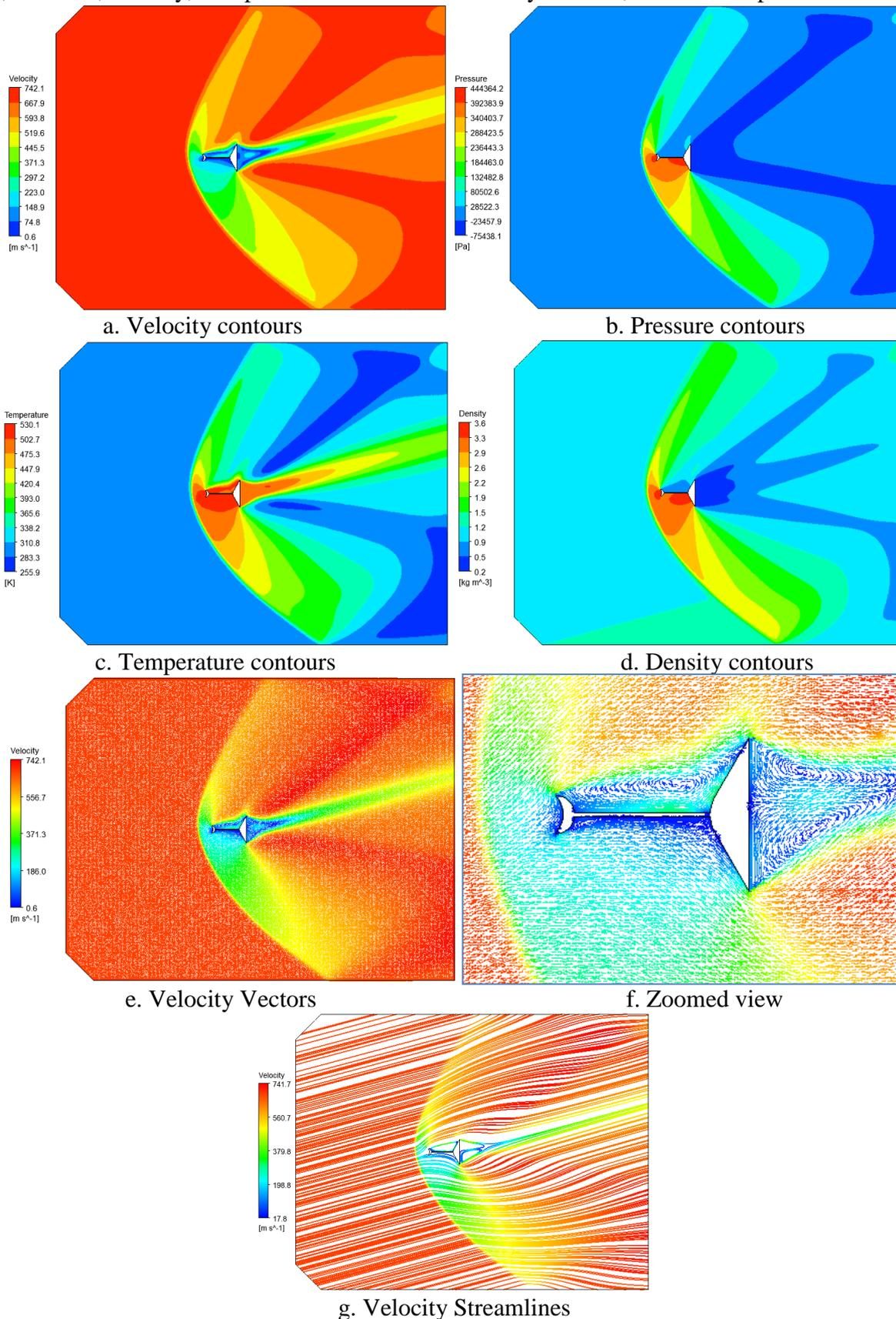
**Fig. 3 : Concave spike blunt nose fluid behavior for 2 Mach speed and 15 deg AOA**
