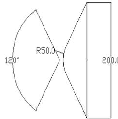
**Fig. 1 : Blunt body without spike configuration**
