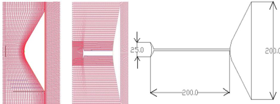
**Fig. 2 : Meshed model for Blunt nose, Concave and concave spike configuration**
