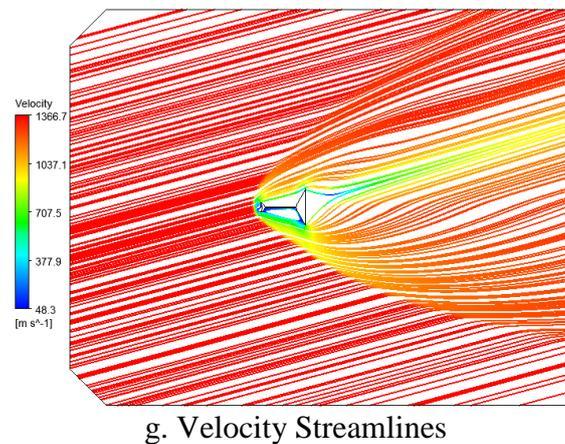
**Fig. 4 : Concave spike blunt nose fluid behavior for 4 Mach speed and 15 deg AOA**
