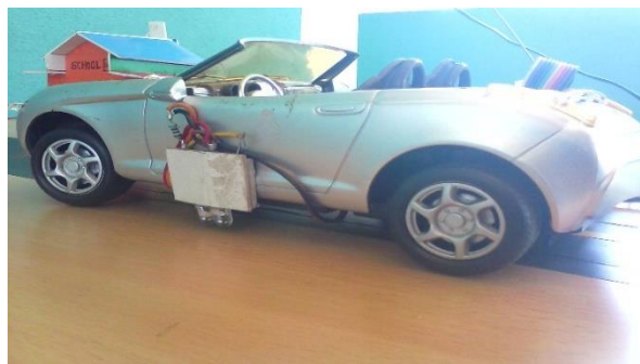
Figure 11. Steep edge detection by IR LED sensor
